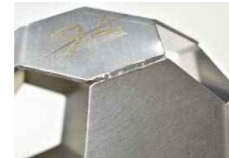
Laser welding of stainless steel (SUS) sheets
