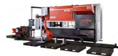
High-accuracy bending robot system HG-1003ARs
