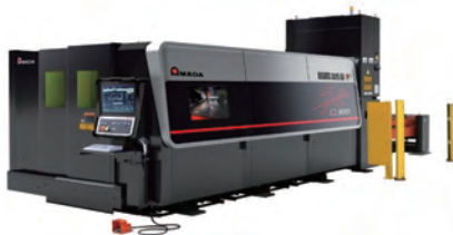
Fiber laser machine with 3-axis linear drive technology REGIUS-3015AJ
