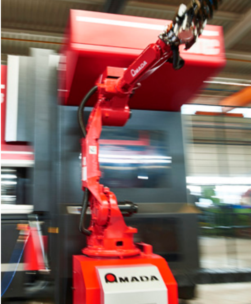
The robot arm is at the heart of the new AMADA HG 1003 ARs which runs around the clock without the need for additional staff.
