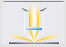
The cutting process is constantly monitored for factors that cause processing defects, such as piercing or plasma, in order to support continued reliable processing.
