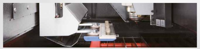
The optional nozzle changer can automatically change to the required nozzle for specific cutting operations. Eight different nozzle stations allow continuous processing of thin to thick sheets without interruption.
