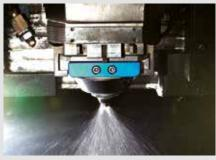
AMADA's original Water-Assisted Cutting System (WACS) uses a fine spray mist when cutting thick material to suppress material overheating, thereby reducing cutting defects and enabling thinner web widths during part nesting. The ultimate benefit is improved material utilisation and stable processing.
