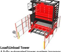
A fully automated tower system incorporating multiple raw material and finished parts pallets to allow continuous scheduled processing. Parts and material can be loaded\unloaded without interrupting the laser cutting cycle.
