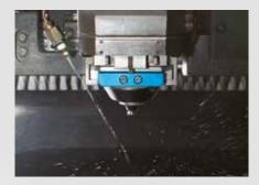
Before piercing a thicker sheet, oil is sprayed on the material to prevent spatter buildup, improve pierce quality, and achieve stable processing.
