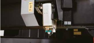
The HS capacitance sensor is constructed to reduce the effect of plasma and adopts a high frequency (MHz) band that is less susceptible to effect of noise, which maintains the gap between the material and laser head during high speed processing for stable cutting.
