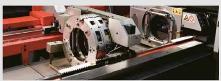
The optional Rotary Index unit can handle rounds, squares, rectangles, channels and angles. The Rotary Index unit substantially reduces the time to switch between flat sheet cutting and tube, angle or section cutting. The Rotary Index unit enables the setup of tubes, angles and sections outside the machine, freeing up the 2 standard cutting pallets for sheet material cutting. The setup time is sharply reduced as a result.
