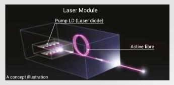
The construction of the fibre laser oscillator and optical transport of the laser beam is less complex than a  $\rm CO_2$  system. This drastically reduces the maintenance requirements of the oscillator and optical parts.
