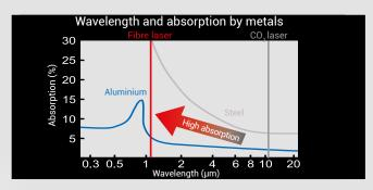
The fibre laser has a shorter wavelength and is 3 to 4 times more easily absorbed than traditional CO<sub>2</sub> lasers.
