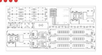
Material: Galvanised Steel, 1.6 mm Dimension: 1830 x 915 mm Number of part types: 11 Total number of parts: 27
