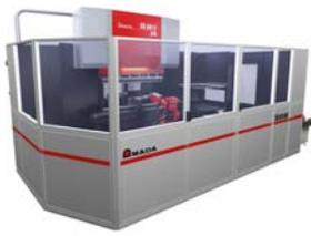
More than just loading and unloading: The automatic robotic system within the AMADA EG-6013 AR bending cell performs a wide range of tasks.
